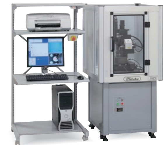
Model: MLP-2 (360-degree measurement model) Measuring range: XYZ = 120mm X 90mm X 130mm AF (R) = 40mm, AZ (θ) = 360° Scale resolution: XYZ = 0.1µm, 0.1µm, 0.1µm AF (R) = 0.01µm, AZ (θ) = 0.001° Applications: precision gears, endmills, punches, molds for connectors, etc.
